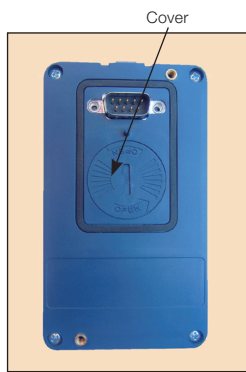
Figure 28: Keypad battery cover to access battery
