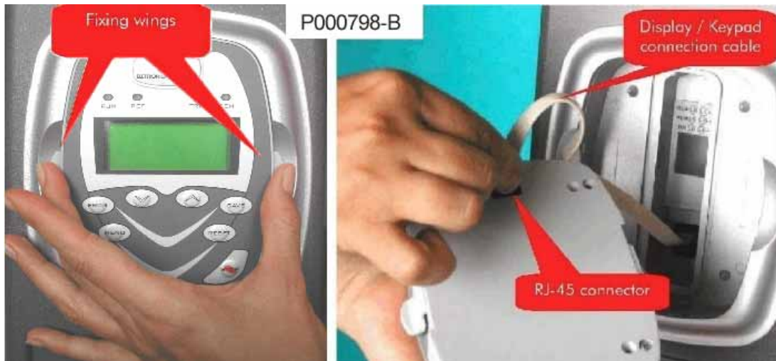
Figure 17: Removing the display/keypad.
