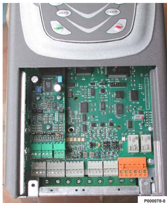
Figure 25: Encoder board fastened to its slot.
