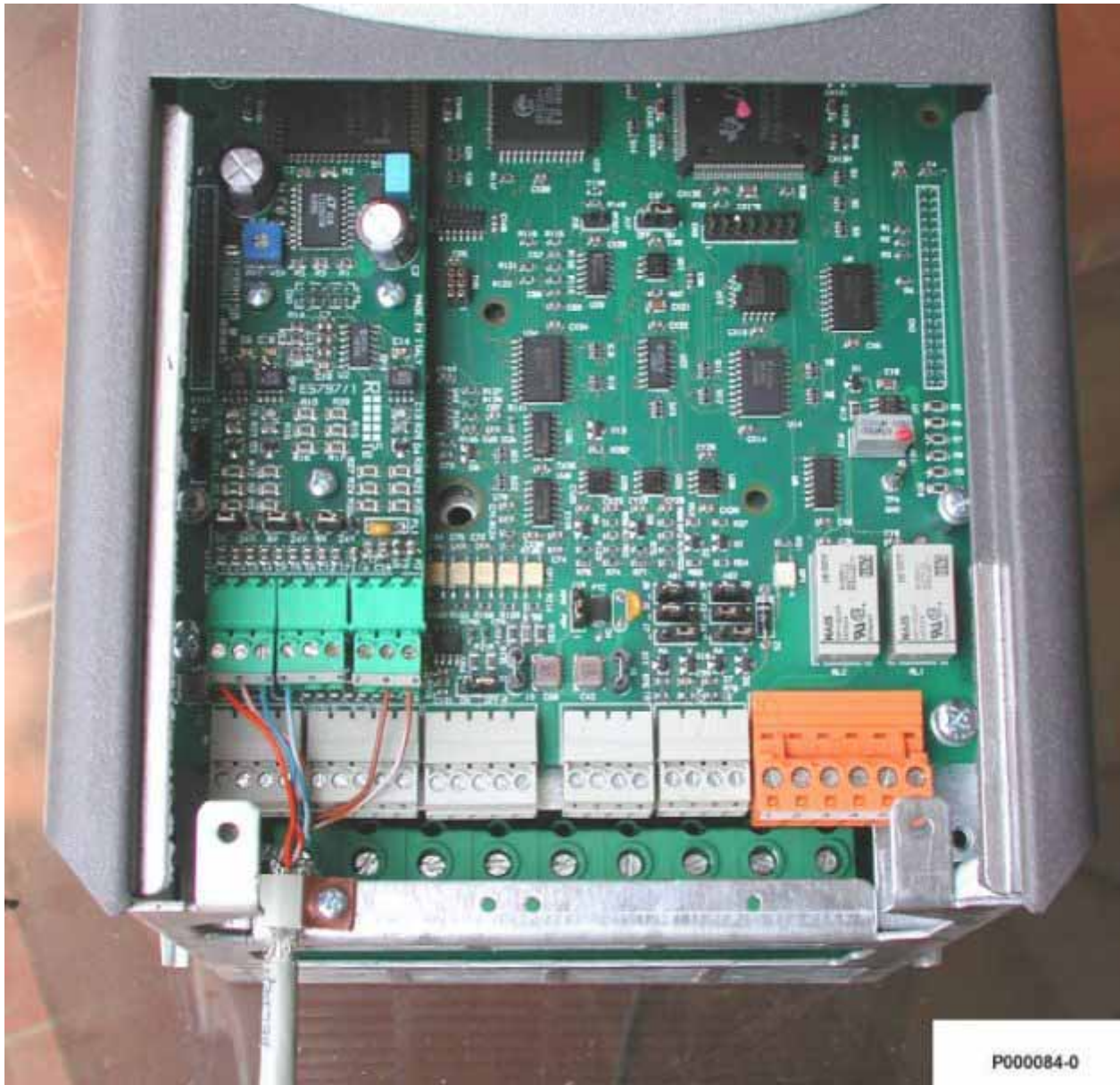
Figure 31: Wiring the encoder cable.
