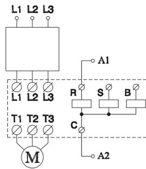
Set Ramp-Up and Initial Torque adjustments for best start-up function. Adjust brake torque to reach a complete stop after each working cycle
