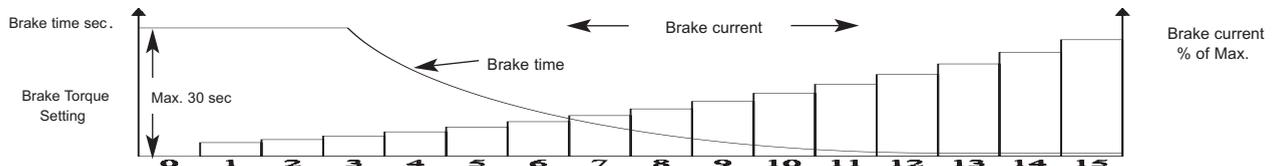
When the Brake current is set it is actually a DC voltage that is adjusted. The current is therefore depending on the ohmic resistance of the windings and the actual connection of the motor (Delta).
