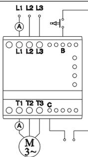
The motor speed is detected by sensing the DC brake current. As this controller can operate a wide range of motors with different wiring configurations, the ohmic resistance of the actual motor has a wide range, it is therefore necessary to adjust the "Brake Torque" (DC Brake current) to achieve correct function in the actual application.
