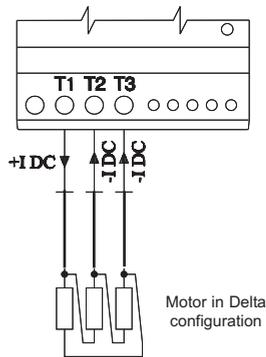
To achieve maximum brake torque the DC current is applied on all 3 motor windings. Direction of current is from T1 to T2 and T3.
