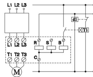
If the application only can accept a low braking torque below the sensing range of the stop detection it is possible to connect an external "delay on" operate timer to the Brake control input.
